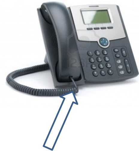
Connect to ICRI's 4-wire audio I/O port
